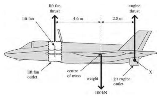
(a) (i) Calculate the moment caused by the weight of the aircraft about the point **X**.
