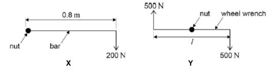
What is the minimum length l of the wrench which would be needed for him to loosen the nut?
