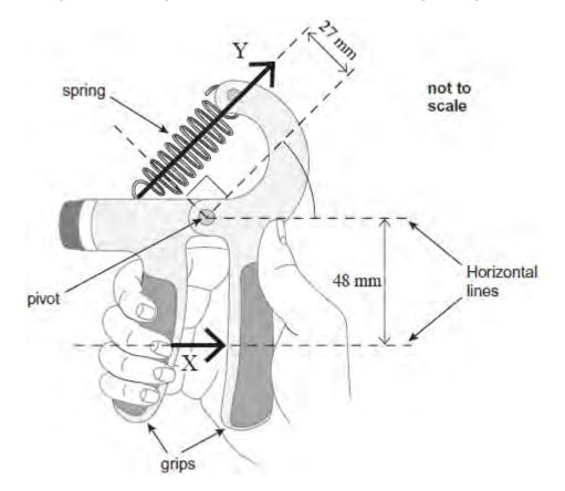
The diagram shows the gripper being squeezed. In this situation, the gripper is in equilibrium. The force produced by the fingers is equivalent to the single force  ${\bf X}$  of magnitude 250 N acting in the direction shown above. A force,  ${\bf Y}$ , is exerted by the spring which obeys Hooke's law.
