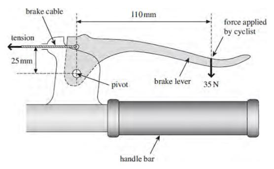
(i) Calculate the moment of the force applied by the cyclist about the pivot. State an appropriate unit.
